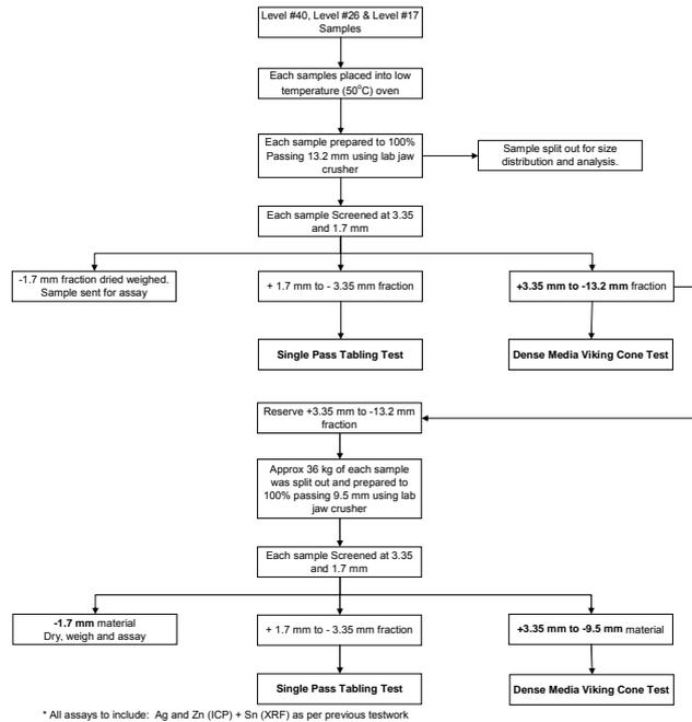
Fig. 4: Flowsheet for Piriquitas continuous gravity recovery test work
