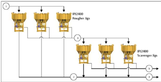
Fig. 8: Simplified PFD of Gekko pre-concentration process at Pirquitas
