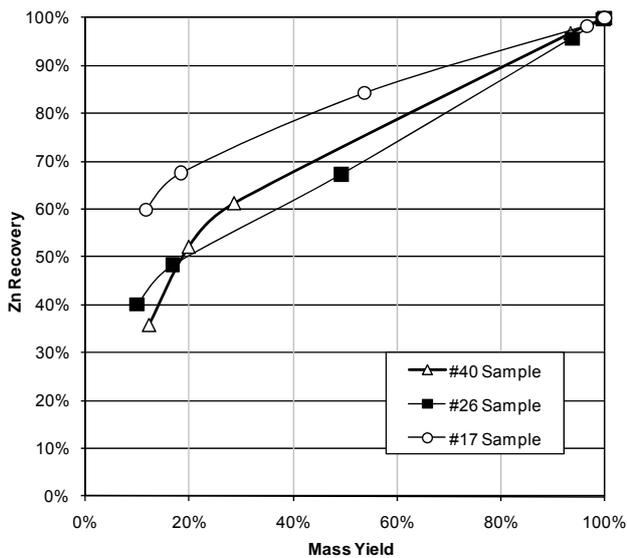
Fig. 7: Zinc recovery versus mass yield from Gekko test work
