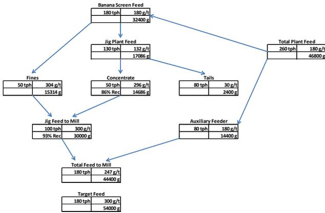
Fig. 11: Mass balance around IPJ circuit
