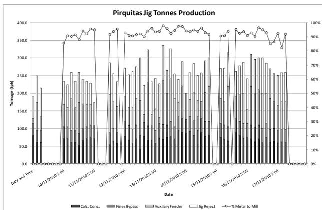
Fig. 12: Tonnes distribution in feed to the Pirquitas milling circuit
