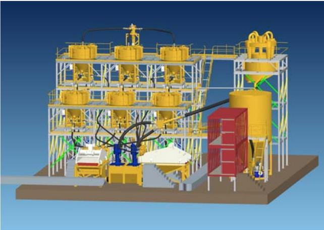
Fig. 9: 3D Model of Pirquitas two stage gravity concentration plant
