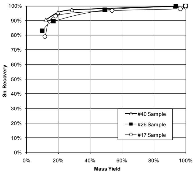
Fig. 6: Tin recovery versus mass yield from Gekko test work
