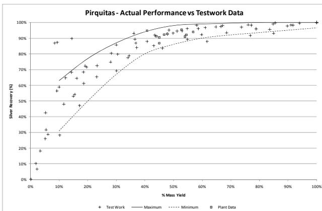
Fig. 14: Silver recovery versus mass yield for test work versus plant data
