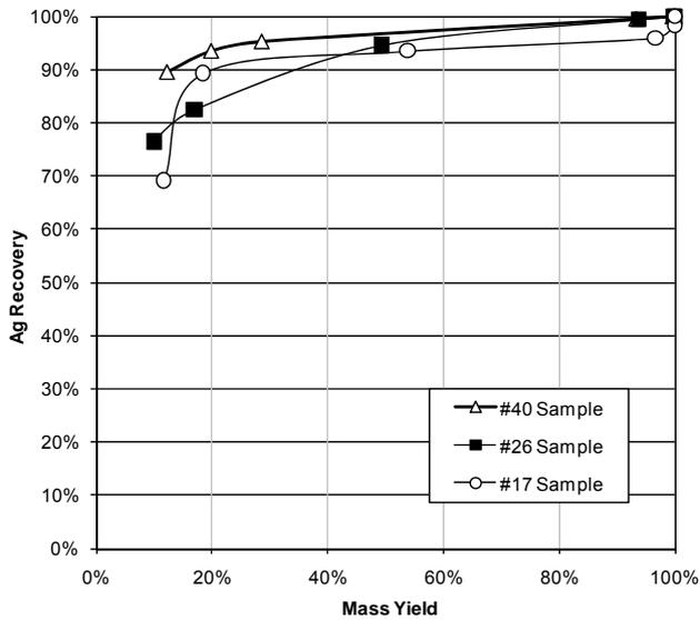
Fig. 5: Silver recovery versus mass yield from Gekko test work
