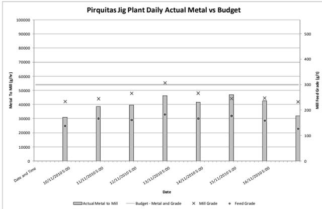
Fig. 13: Silver grade and metal feed rate to the Pirquitas milling circuit
