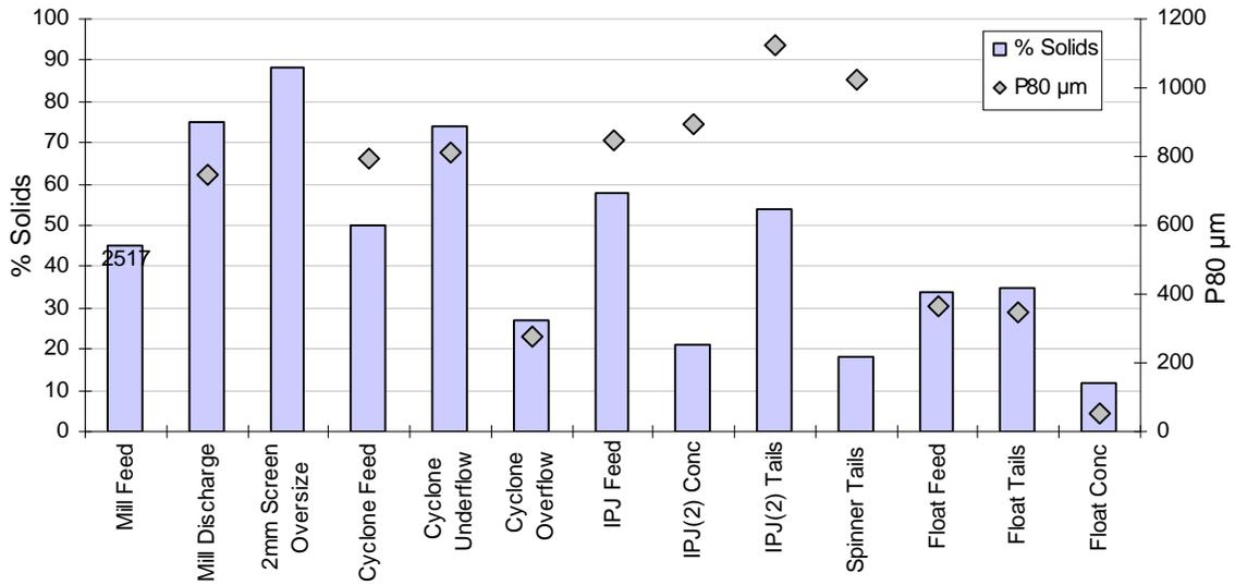
**Figure 2:** %Solids and Grind size measured in process streams
