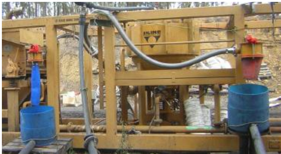
Figure 3. Skid mounted 5 tonne/h GICS on site
