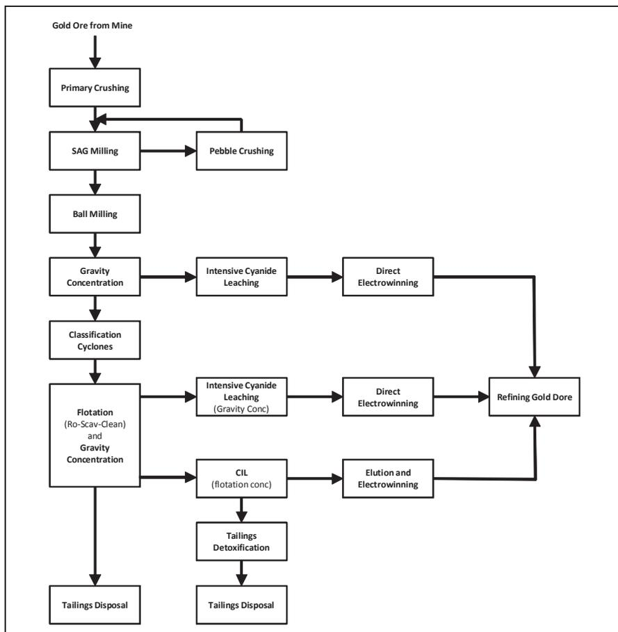
FIG 1 - Simplified gold recovery process block flow diagram.
