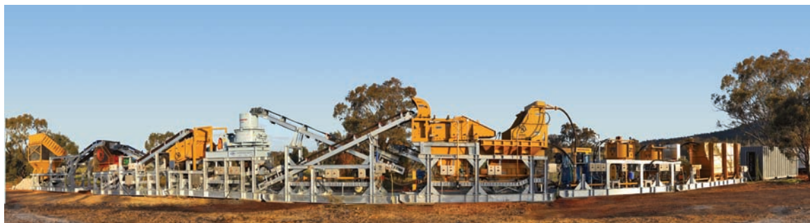
FIG 10 - Python 200 unit showing, from left to right, secondary crusher, secondary and tertiary screens and InLine Pressure Jigs in closed circuits.
