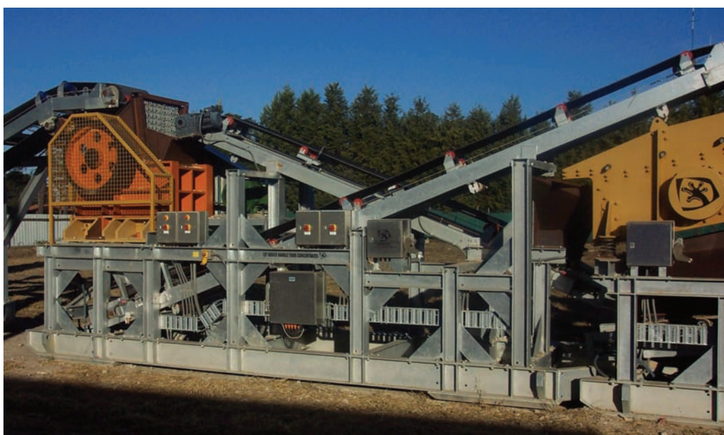
FIG 9 - Python 200 unit showing primary screen and jaw crusher in closed circuit.
