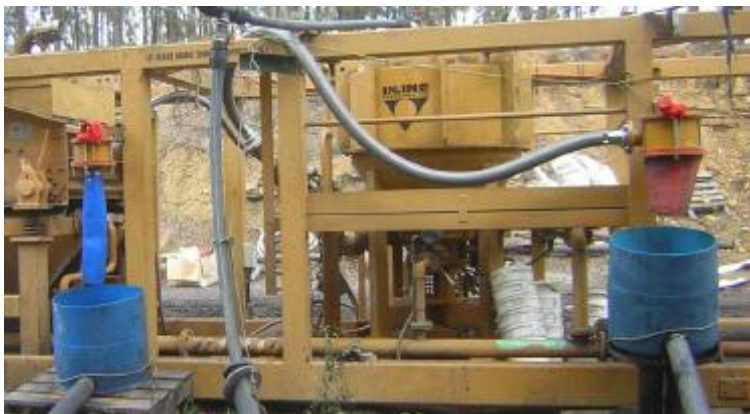
Figure 3. Skid mounted 10 tph Gekko IPJ Coal Separator on site
