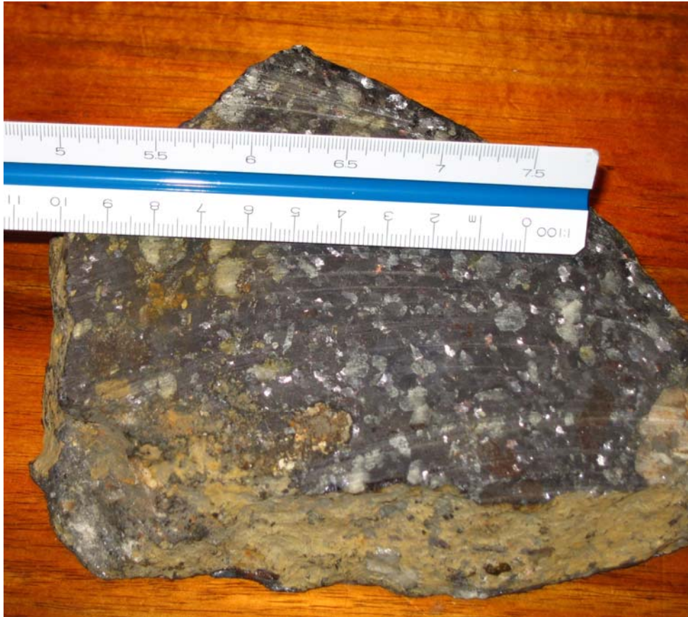
Figure 9: Sample of Phuoc Son Ore indicating coarse nature of Sulphides
