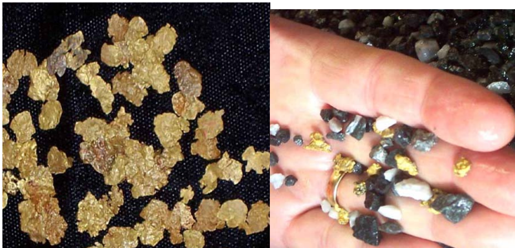
Figure 2: Free gold recovered from a milling circuit (Left) versus HPGR (Buerger, 2006).
