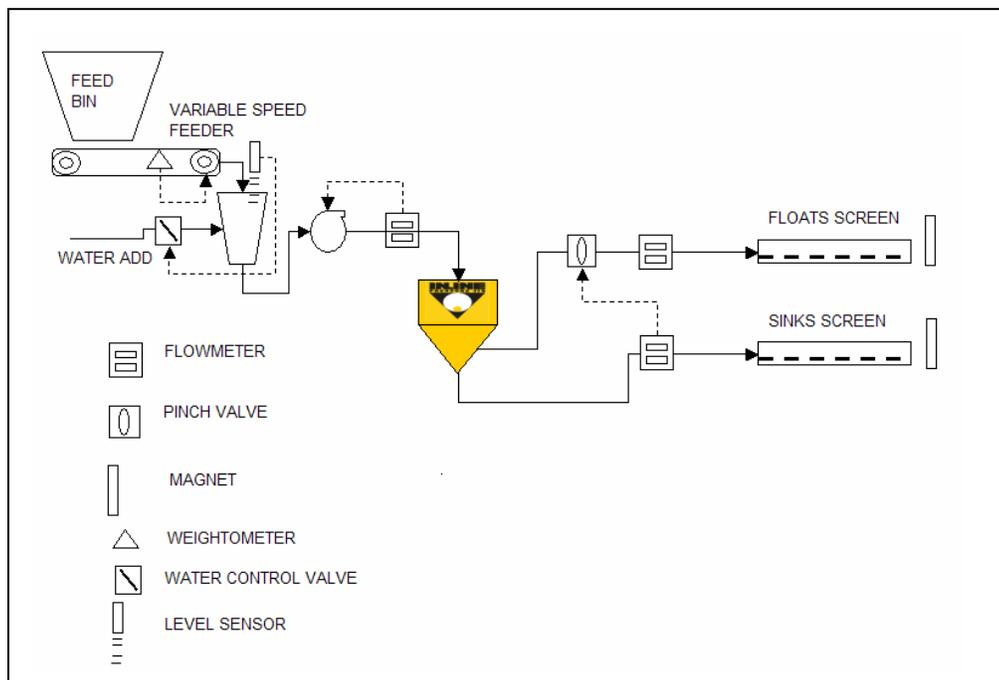
Fig 6: Automation schematic for IPJ plant - Gekko recommendation
