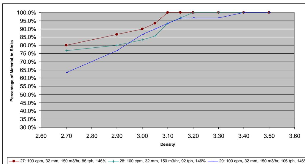
**Figure 10: Partition Curves for 8 mm Tracers at Varying Solids Feed Rates**
