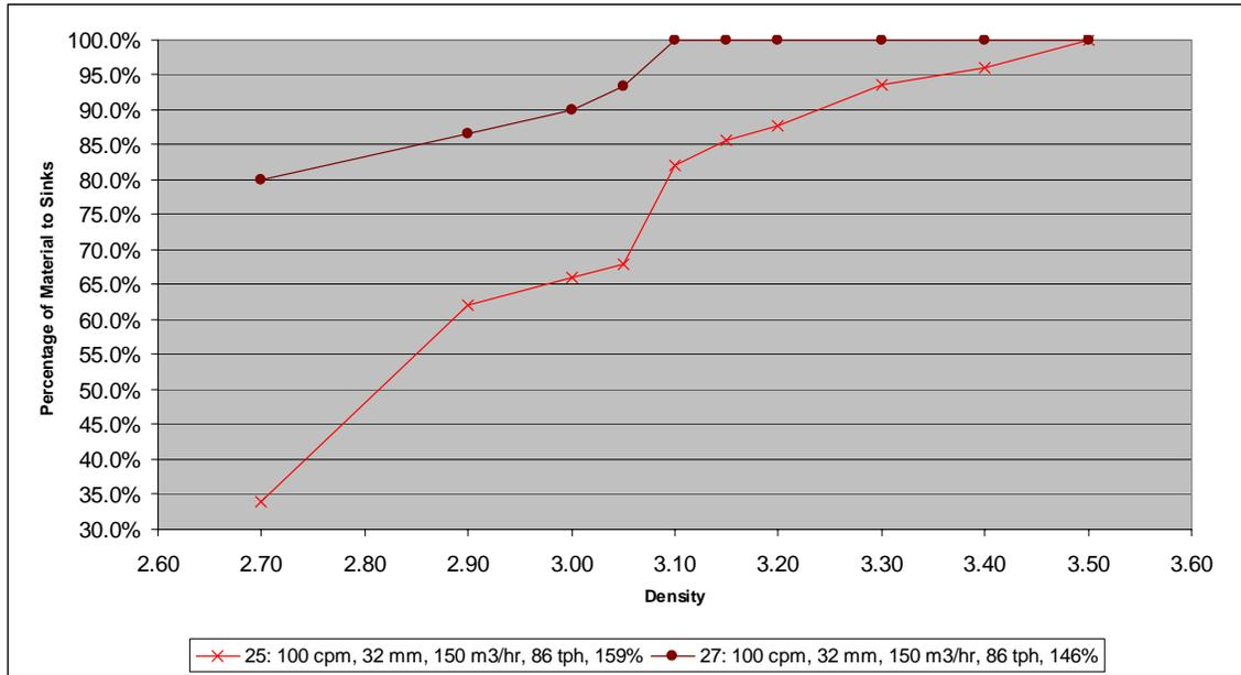
**Fig 9: Partition Curves for Ragging Profiles of 146% and 159% for 8 mm Tracers**
