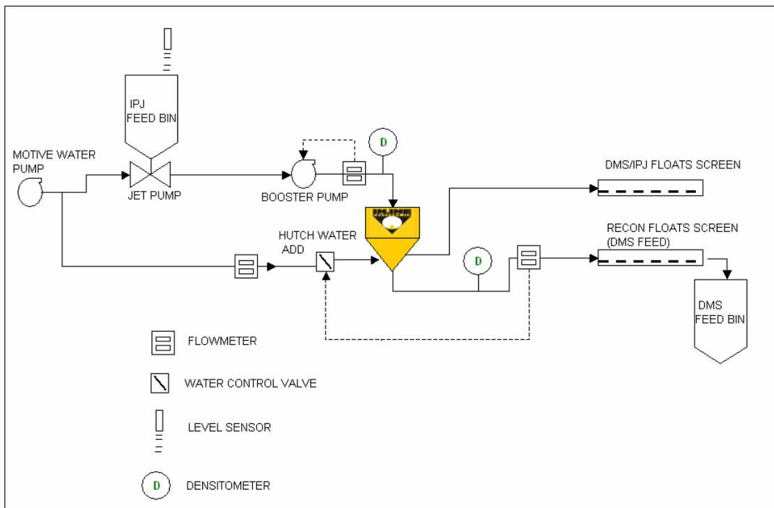
Figure 17: Automation Schematic for IPJ Plant – Namdeb design
