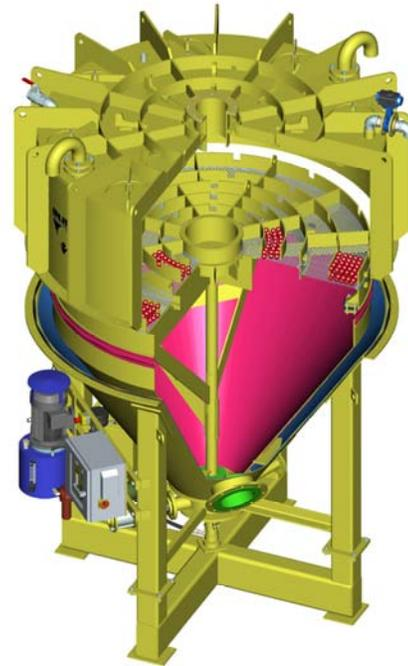
Fig 1: Cutaway Section through IPJ2400
