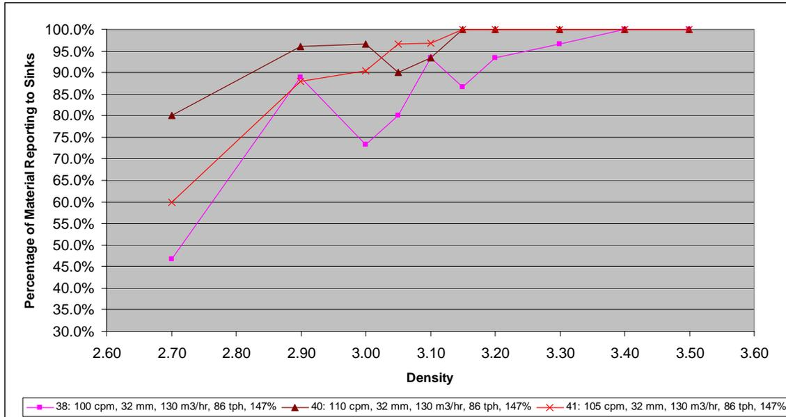
**Figure 14: Partition Curves for Pulse Rates of 100, 105 and 110 cycles/min for 8mm Tracers**
