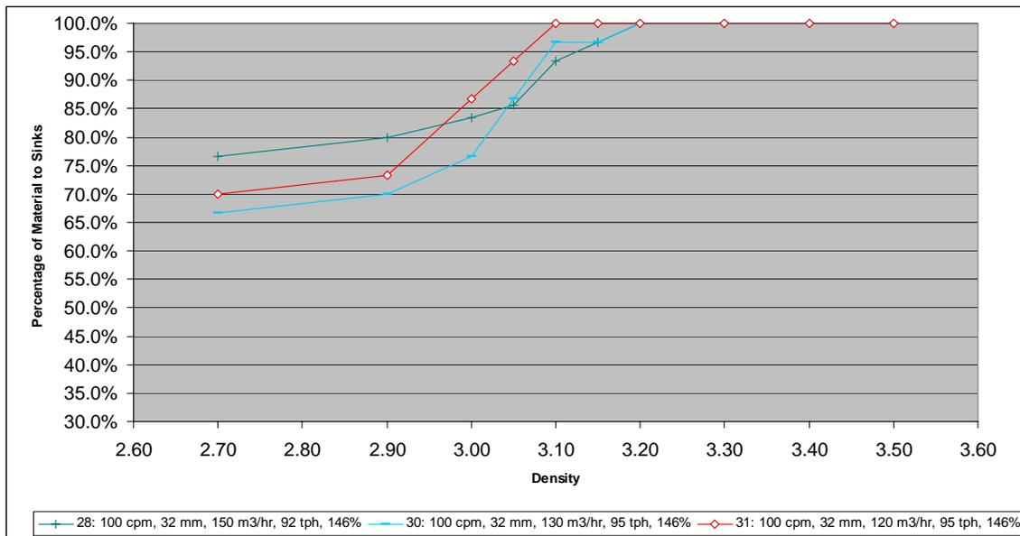
Figure 12: Partition Curves for Volumetric Flow Rates of 150, 130, & 120 m<sup>3</sup>/hr
