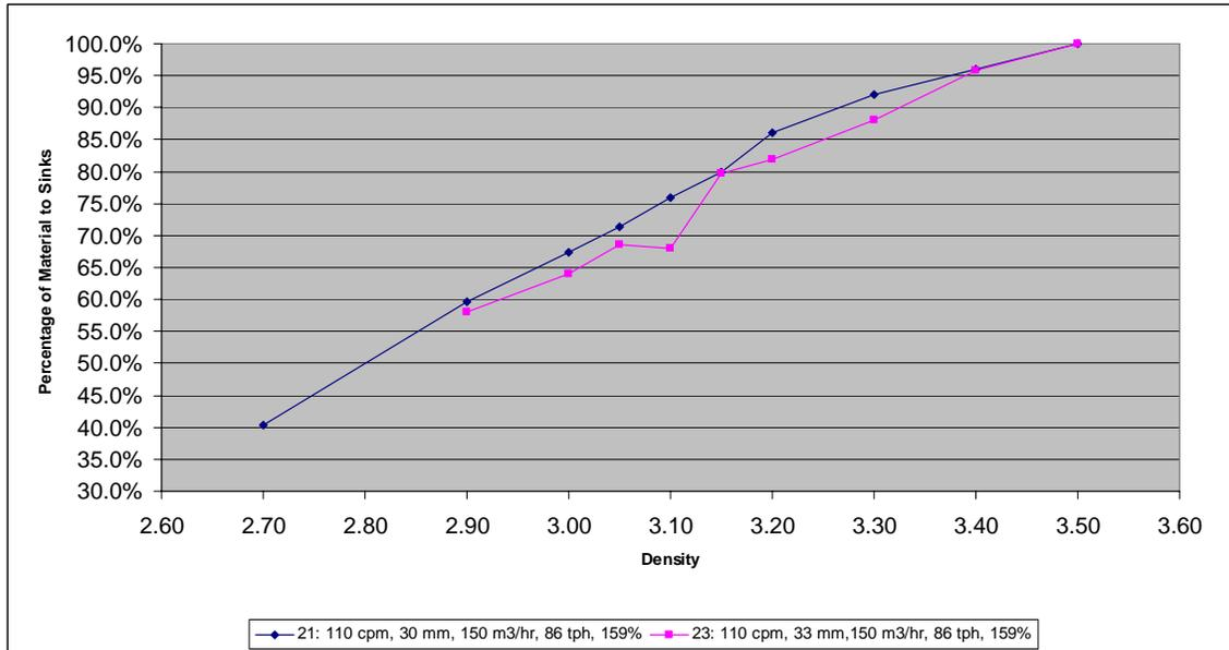
Figure 13: Partition Curves for Stroke Lengths of 30 mm and 33 mm for 8 mm Tracers
