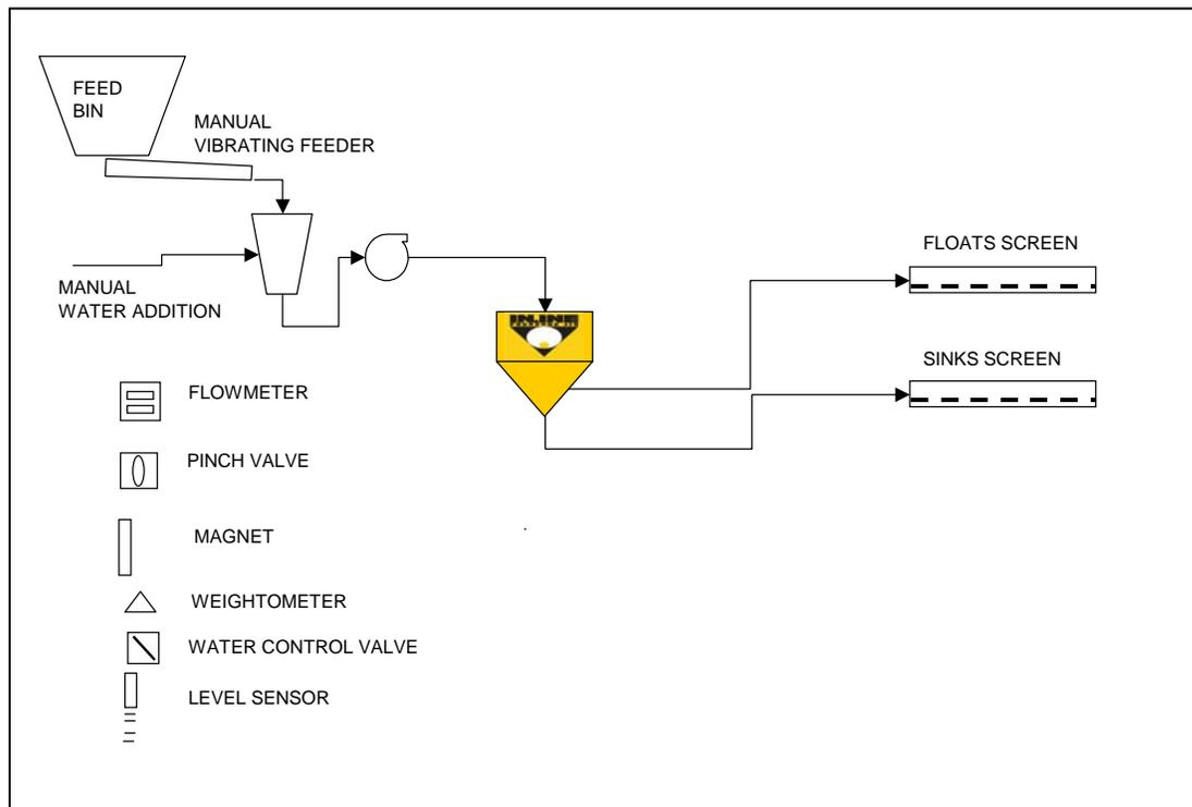
**Fig 5: Automation schematic for IPJ plant as installed**
