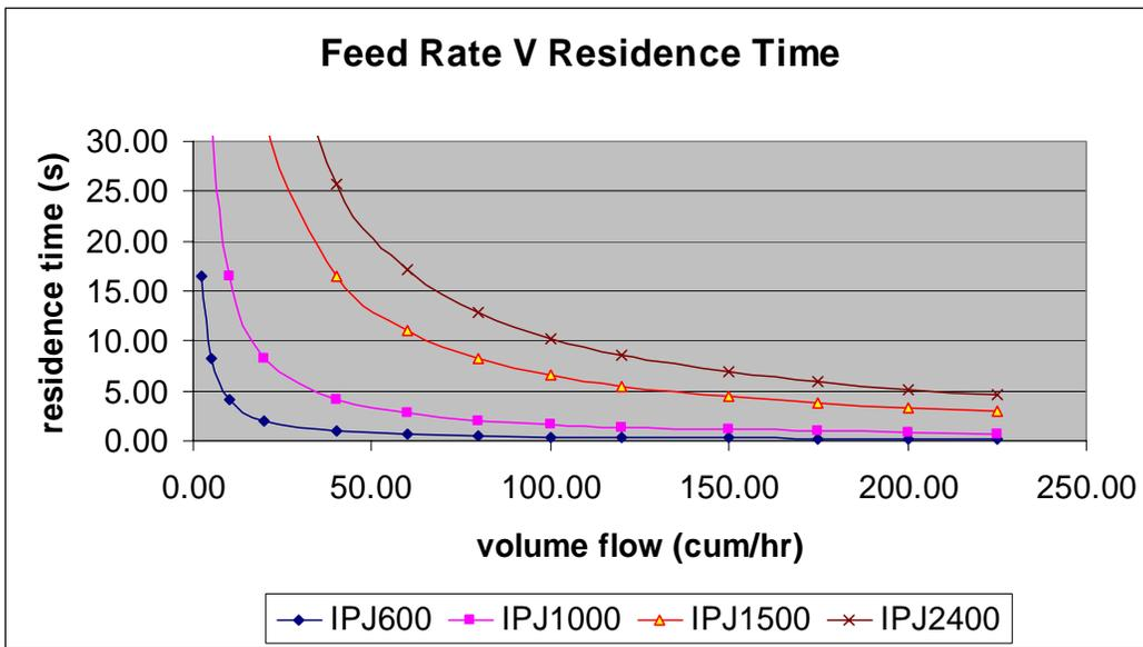
Fig 11: Effect of Volumetric feed rate on IPJ residence time
