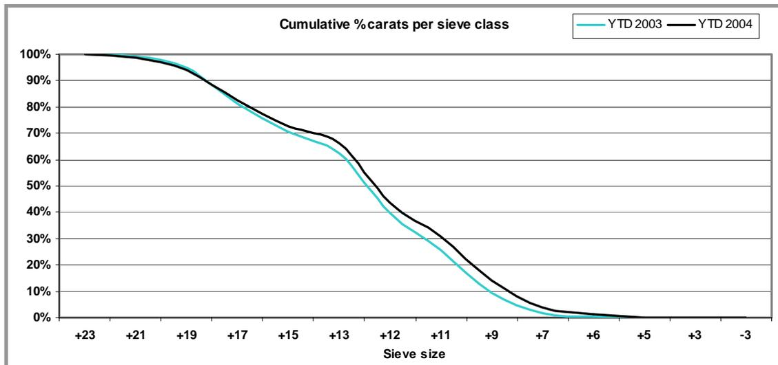
Figure 18: Diamond SFD's prior (2003) and post (2004) IPJ installation
