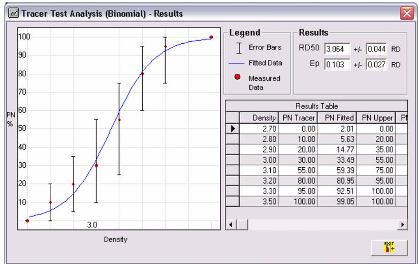
Fig 2: Typical partition curve for density tracer results
