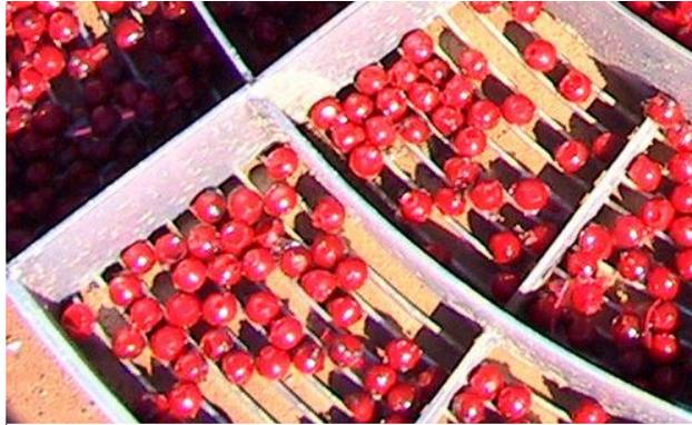
**Fig 8: Synthetic 3.2 sg ragging on IPJ Hutch screen**
