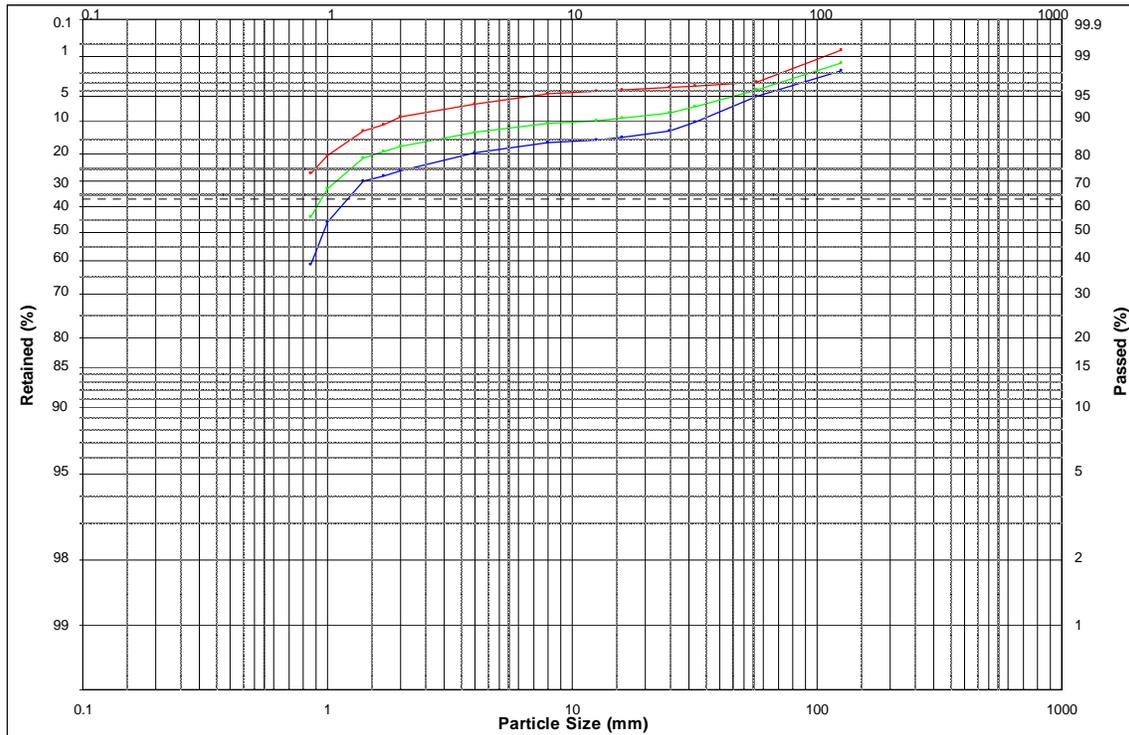
Figure 16: Size Frequency Distribution for DMS Head Feed
