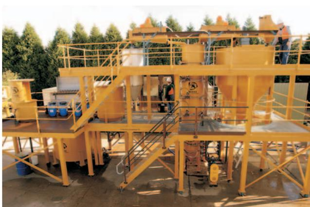
FIG 11 - Picture of the Gekko resin column modular plant, capable of recovering 50 000 oz gold/annum.
