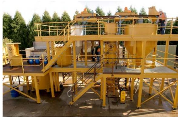
Figure 14: A recently constructed Gekko Resin Column, resin stripping and electrowinning circuit
