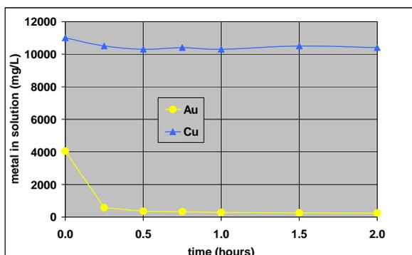
**Figure 12:** Copper/gold Absorption curves for Brown's Creek gold/copper solution
