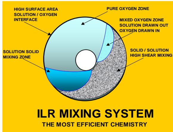
**Figure 2:** ILR mass transfer zones within the reactor drum
