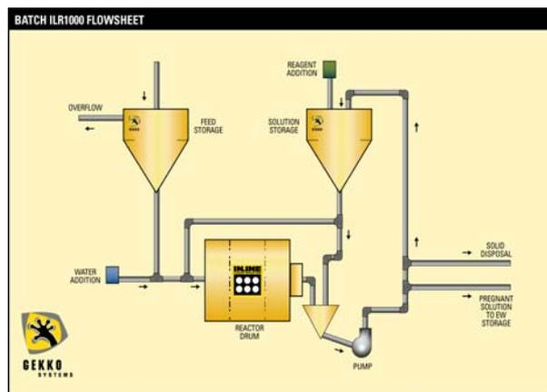
Figure 1: Gekko Inline Leach Reactor
