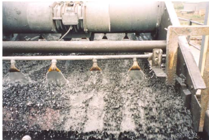
Figure 7. shows material flowing to discharge without screening due to very high density feed.
