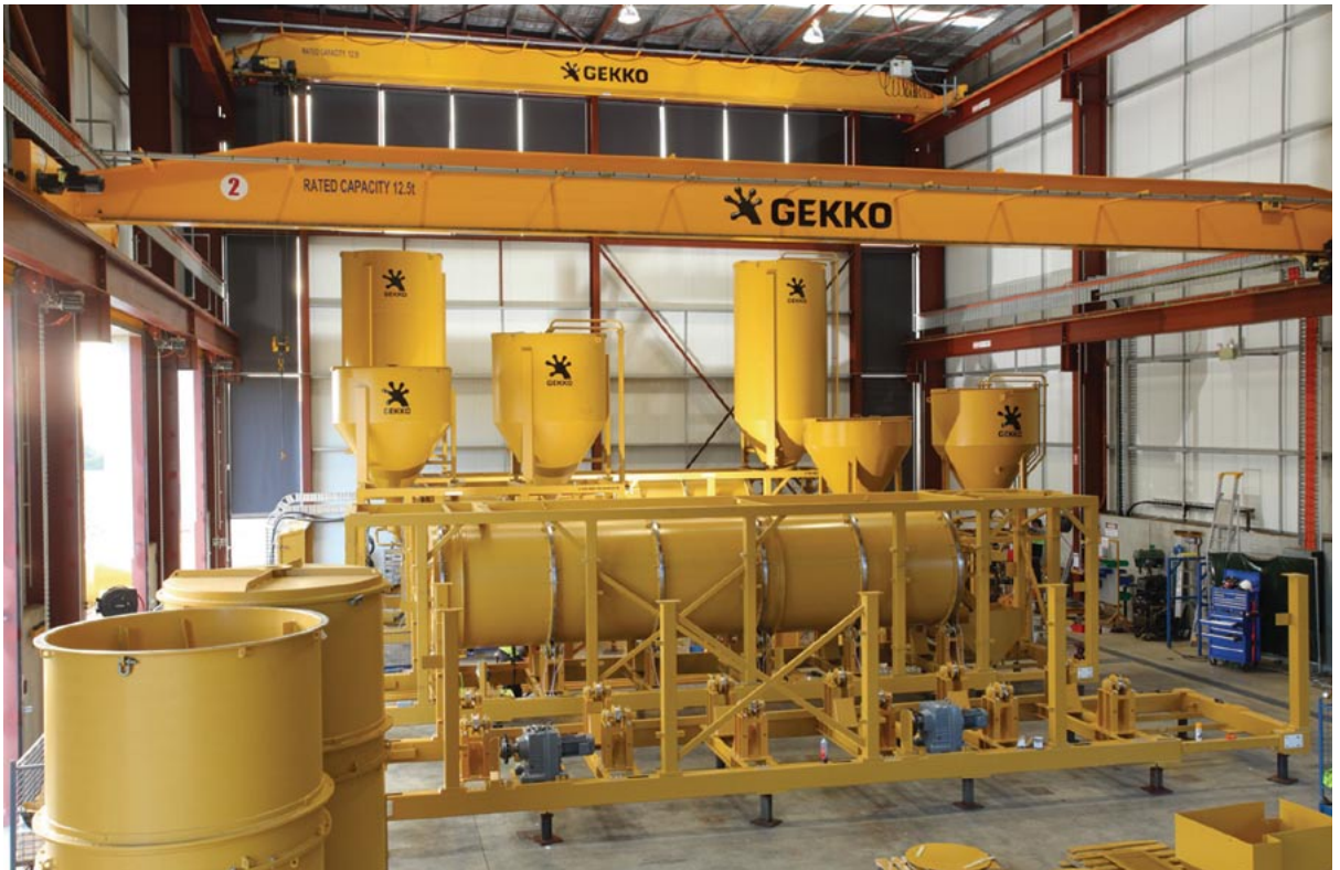
Verninskoye, Xstrata, Muriel Mining and Alamos ILRs nearing completion in Gekko's state-of-the-art manufacturing facility
