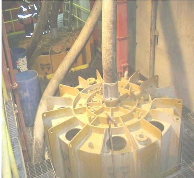
**View of IPJ2400 lid platform showing the feed pipes from the rotating distributor**
