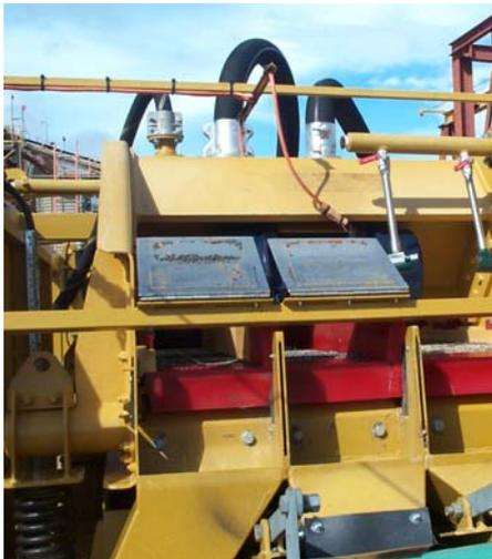
**Figure 7:** Gekko Magnet Tracer Recovery System for Argyle Pilot Plant
