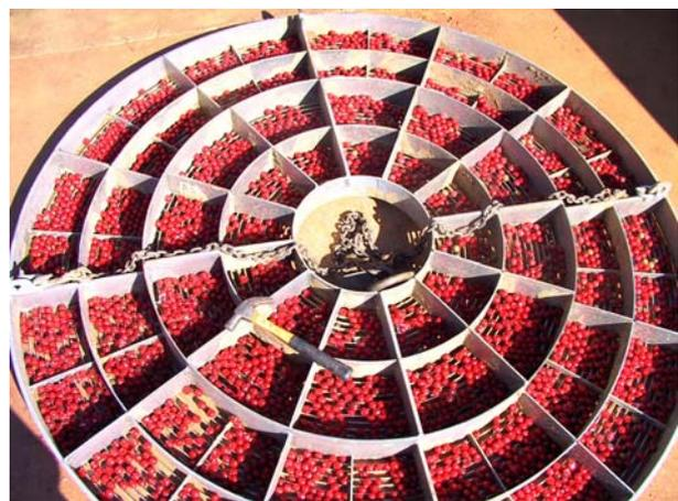
**Figure 1:** A mono-layer of 3.2 S.G ragging installed at KDC's Ellendale project
